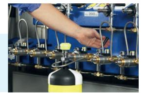
OUR BREATHING AIR ADAPTERS WERE DEVELOPED FOR FAST CONNECTION OF BREATHING AIR CYLINDERS.
