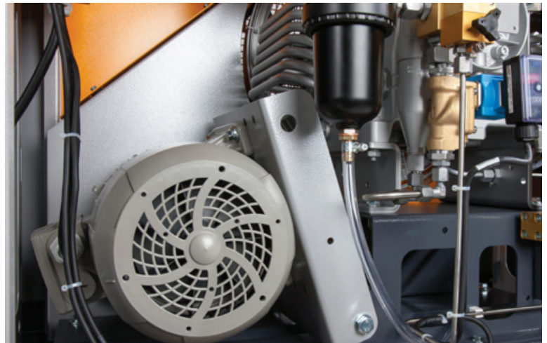
PE-HE: V-belt adjustment is likewise unnecessary in this horizontal model by use of a belt tensioning device.
