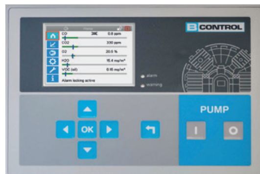
Display showing limit values in compliance with DIN EN 12021:2014
