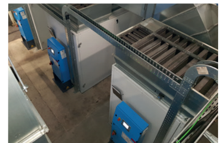
BAUER high pressure compressors deliver the necessary pressure to the presses.
