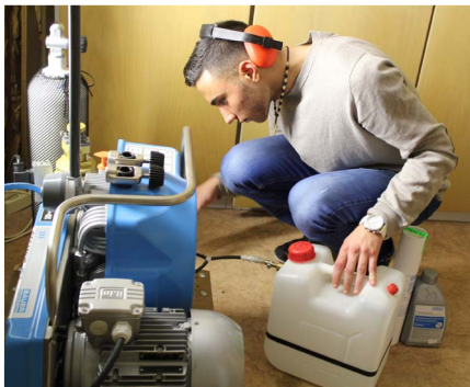
Assistant Issa Kayed replacing a filter cartridge on the OCEANUS
