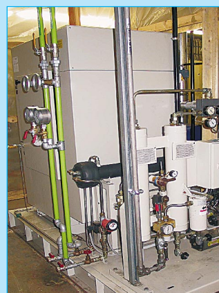
MP-compressor modell B12.4-4 with regeneration dryer, activated carbon adsorber and heat exchanger ■
